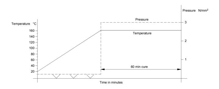
Figure 2 – Conditions for press procedure
